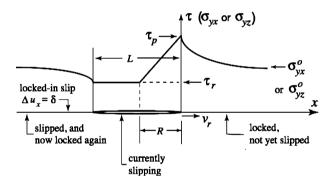
Figure 14 Geometry and parameters of the nonsingular slip-weakening slip-pulse model from RICE *et al.* (2005).
