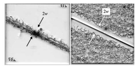
The Homalite plate on the left has a damage band of width 2w centered on the fault. The plate on the right has an undamaged band of width 2w centered on the fault.
