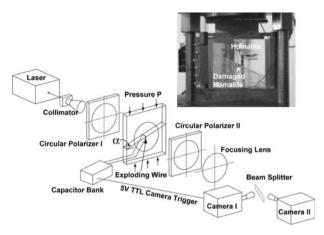
Schematic diagram of apparatus used to take a series of high-speed photographs of dynamic ruptures on premachined faults in photoelastic Homalite and polycarbonate plates. The inset shows a sample in the loading frame used to apply uniaxial stress *P*.
