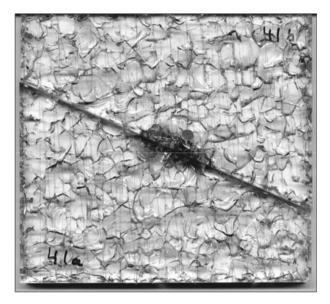
Fracture-damaged sample produced by first scoring both sides of the Homalite plates with a razor knife and then submersing in liquid nitrogen for 45 seconds. The center of the fault plane has been darkened by the explosion that nucleated rupture.
